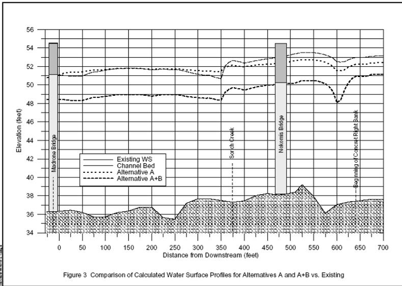
**Figure 3.** Comparison of Calculated Water Surface Profiles for Alternatives A and A+B vs. Existing
