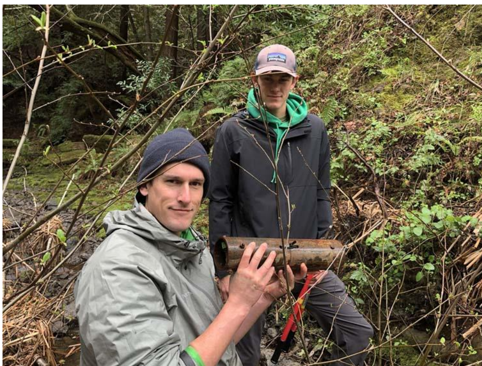
Board member Parker Pringle (left) and Drake High student Logan Smith with a DO logger inside its protective casing, just before it was installed. Every effort is made to hide the loggers to prevent vandalism and theft. Photo by Sandy Goldman
