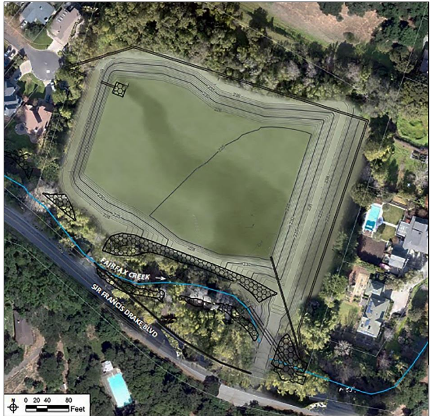
Plan view of the conceptual design for a detention basin/flood plain at the former Sunnyside Nursery growing grounds in Fairfax. If flooding in downtown Fairfax were imminent, a gate on Fairfax Creek would be closed and water would flow into the basin over the armored sill along the southern edge of the basin. A low-level channel would remain open so that some flow would continue in Fairfax Creek even as the basin filled. This drawing is a simplified version of Figure 2-2 in the draft EIR, available on the project website, prepared by Marin County Flood Control District, Geomorph Design, Walls Land+Water, and Stetson. Detailed designs will be developed when environmental review is complete.
