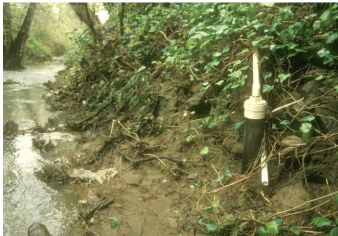
Well heads close to the creek can directly lower water levels and affect aquatic wildlife; wells further away have an unknown effect on the creek, but deplete the aquifer that feeds the creek throughout the dry season. Photo by Lou Vaccaro
