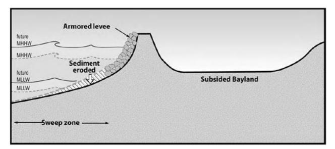
**Traditional Levee:** A traditional levee allows waves to reach the levee at full height. The detailed studies show that traditional levees must be twice as high as the impermeable berm of a horizontal levee to provide the same level of flood protection. Graphic courtesy The Bay Institute and ESA/PWA.
