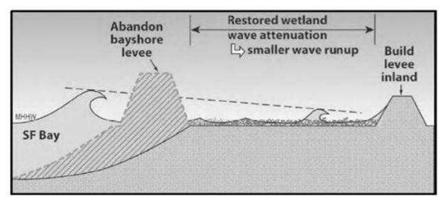
**Marsh and Levee:** An alternative without the freshwater swale and brackish marsh provides wave attenuation, but not the resilience to sea level rise. It is an option if a horizontal levee is not feasible. Even where there are no bayshore levees, this could be an option to reduce flood risk as sea level rises. Graphic courtesy The Bay Institute and ESA/PWA.
