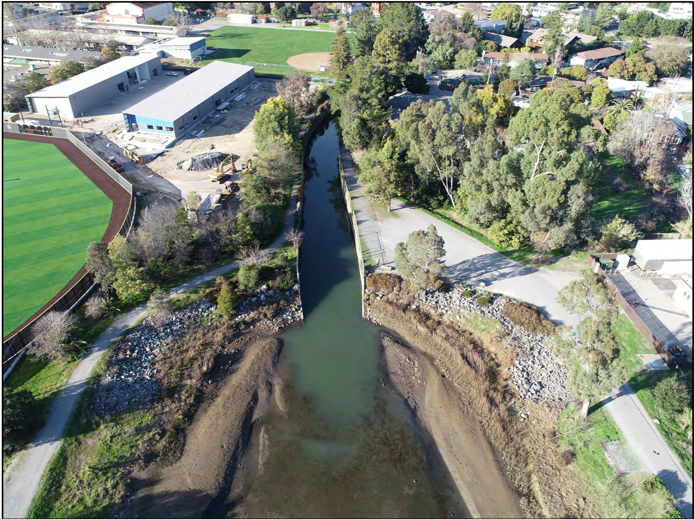
EXISTING CONDITIONS DATE OF FLIGHT: 5 FEB 2020 AT LOW TIDE (~0.4' NAVD88) (SEDIMENTATION IN THE EARTHEN CHANNEL DOWNSTREAM FROM THE CONCRETE CHANNEL PREVENTS TIDE LEVEL IN THE CONCRETE CHANNEL FROM REDUCING BELOW RIFFLE ELEVATION (APPROX. 1.7' NAVD88, SURVEYED FEB 2020).
