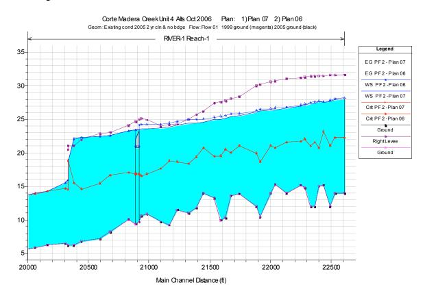
**Figure 3.** *Plan 06/07.* Comparison of calculated water surface profiles for PF2 (3,250 cfs) in the Unit 4 reach for 2005 existing conditions geometry with the existing Lagunitas Road Bridge intact (g05, Plan 06) and for 2005 existing conditions geometry with Lagunitas Road Bridge removed (g06, Plan 07).
