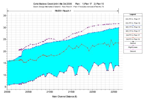
**Figure 20.** Plan 17/15. Comparison of calculated water surface profiles for PF4 (4,700 cfs) in the Unit 4 reach for the Design Alternative II Variant 2 plan (g14, Plan 15) and the Design Alternative II Variant 3 plan (g16, Plan 17).
