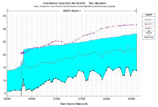
**Figure 29.** Plan 26. Flood water surface elevation profile for PF1 (3,200 cfs) under recommended Alternative I (g09, Plan 26).
