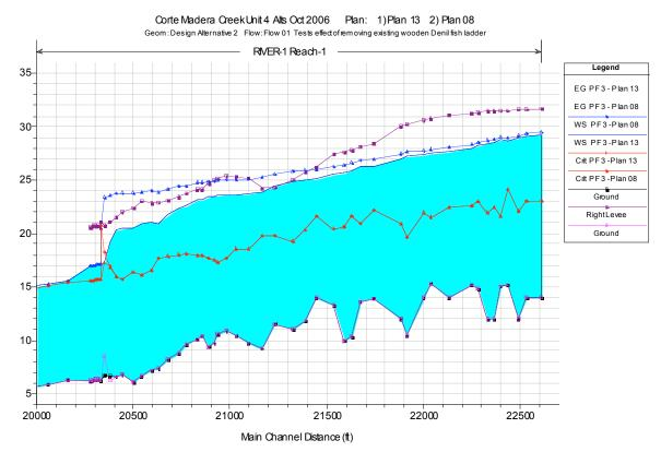
**Figure 12.** *Plan 08/13.* Comparison of calculated water surface profiles for PF3 (4,100 cfs) in the Unit 4 reach for the Baseline (Existing Conditions) Alternative (g07, Plan 08) and the Design Alternative II test (g12, Plan 13). Comparison of Plan 08 and Plan 13 demonstrates the isolated effect of only removing the existing grade control fish ladder structure and locally redistributing some of the existing rip-rap immediately upstream from the structure.
