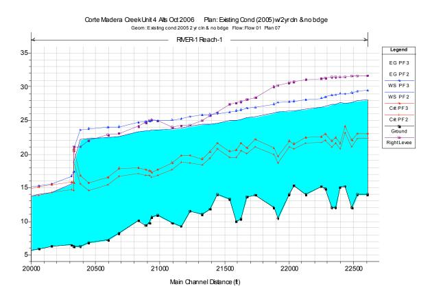
**Figure 4.** *Plan 07.* Comparison of calculated water surface profiles for PF2 (3,250 cfs) and PF3 (4,100 cfs) in the Unit 4 reach for 2005 existing conditions geometry with the Lagunitas Road Bridge structure removed (g06, Plan 07). The geometry file includes the existing wooden Denil fish ladder structure at the Unit 3/Unit 4 transition.
