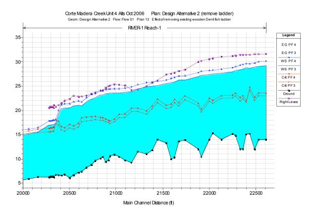
**Figure 13.** Plan 13. Comparison of calculated water surface profiles for PF3 (4,100 cfs) and PF4 (4,700 cfs) in the Unit 4 reach for the initial Design Alternative II test (g12, Plan 13).
