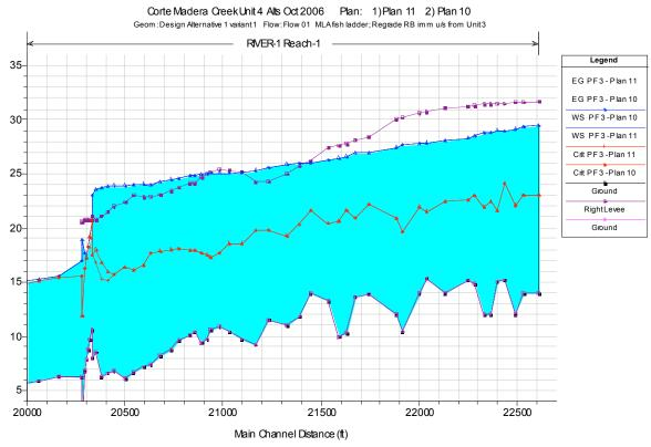
**Figure 9.** *Plan 10/11.* Comparison of calculated water surface profiles for PF3 (4,100 cfs) in the Unit 4 reach for the Design Alternative I test (g09, Plan 10) and the Design Alternative I Variant 1 (g10, Plan 11). Both geometry files include the preliminary replacement fish ladder concept design within the upstream end of Unit 3 concrete channel (MLA, May 30, 2006). Comparison of Plan 10 and Plan 11 demonstrates the
