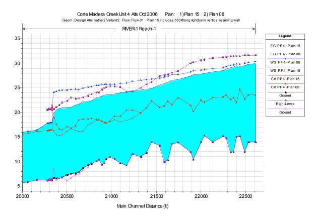
**Figure 19.** *Plan 08/15.* Comparison of calculated water surface profiles for PF4 (4,700 cfs) in the Unit 4 reach for the Baseline (Existing Conditions) Alternative (g07, Plan 08) and the Design Alternative II Variant 2 plan (g14, Plan 15). See Figure 17 for further description of Design Alternative II Variant 2.
