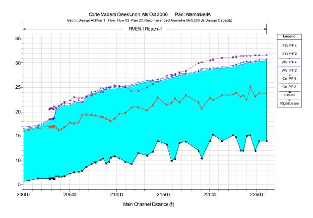
**Figure 30.** *Plan 27.* Comparison of flood water surface elevation profiles for PF2 (5,000 cfs) and PF4 (5,200 cfs) under recommended Alternative IIA (g13, Plan 27).
