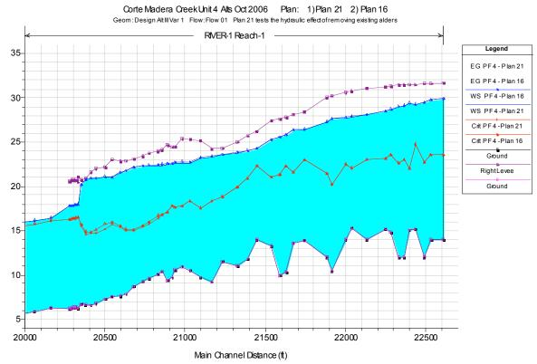
**Figure 25.** *Plan 16/21.* Comparison of calculated water surface profiles for PF4 (4,700 cfs) in the Unit 4 reach for the Design Alternative III Variant 1 (g18, Plan 21).and the Design Alternative III test plan (g15, Plan 16). This comparison tests the isolated hydraulic effect of removing the 27 existing alders along the toe of the bank along a total of 240 lineal ft of Unit 4, and grading down the associated gravel bar bench to the base of the alders.
