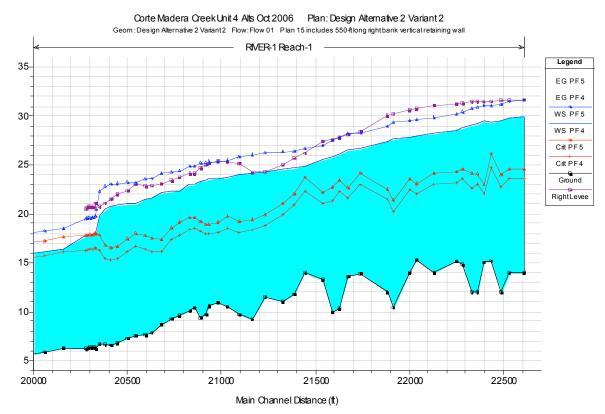
**Figure 18.** Plan 15. Comparison of water surface elevations under Design Alternative II Variant 2 conditions for FP4 (4,700 cfs) and PF5 (5,950 cfs). See Figure 17 for further description of Design Alternative II Variant 2.
