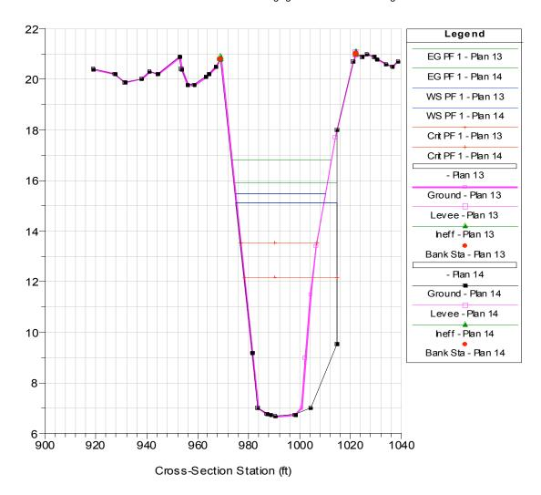
**Figure 14.** *Plan 13/14.* Comparison of cross-section geometry for existing conditions (Design Alternative II test) (g12, Plan 13) and Design Alternative II Variant 1 (g13, Plan 14) at River Station 370+21 ft. The top of the existing sewer siphon pipe concrete encasement at River Station 370+21 ft is at approx. elevation 5.6 ft at Cross-Section Station 1009 ft.
