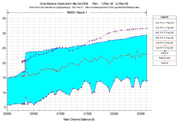
**Figure 6.** Plan 08/09. Comparison of calculated water surface profiles for PF3 (4,100 cfs) in the Unit 4 reach for the Baseline condition (g07, Plan 08) and the Baseline condition with 10-ft widened channel in the vicinity of the Lagunitas Road Bridge (g08, Plan 09). Plan 09 represents replacing the existing Lagunitas Road Bridge abutments with new vertical abutments set back 5 horizontal feet on both the left and right banks (10-ft overall widening between abutments).
