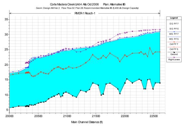
**Figure 31.** *Plan 28.* Comparison of flood water surface elevation profiles for PF5 (5,400 cfs) and PF7 (5,600 cfs) under recommended Alternative IIB (g14, Plan 28).
