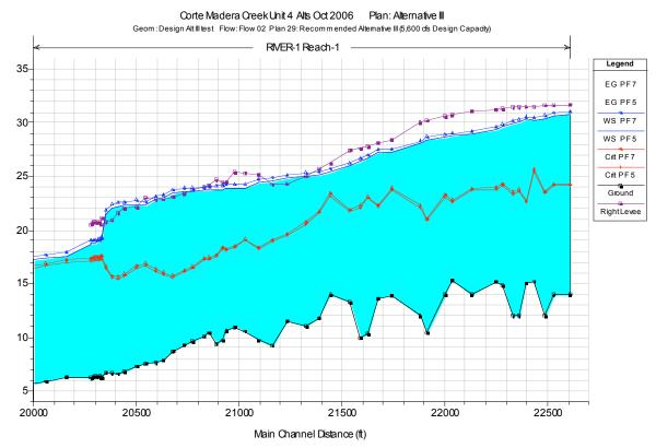
**Figure 32.** Plan 29. Comparison of flood water surface elevation profiles for PF5 (5,400 cfs) and PF7 (5,600 cfs) under recommended Alternative III (g15, Plan 29).
