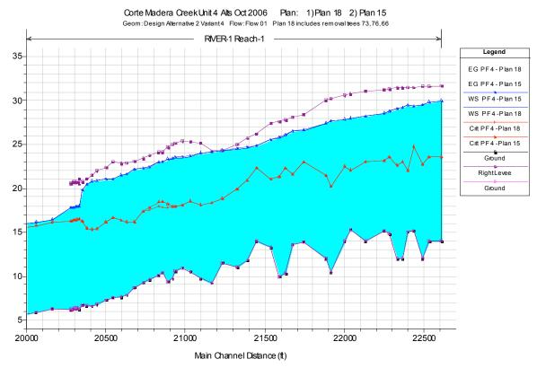
**Figure 21.** Plan 18/15. Comparison of calculated water surface profiles for PF4 (4,700 cfs) in the Unit 4 reach for the Design Alternative II Variant 2 plan (g14, Plan 15) and the Design Alternative II Variant 4 plan (g17, Plan 18).
