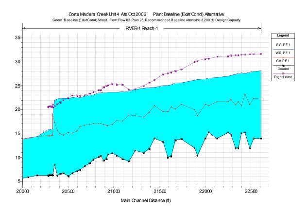
**Figure 28.** Plan 25. Flood water surface elevation profile for PF1 (3,200 cfs) under recommended Design (Existing Conditions) Alternative (g07, Plan 25).
