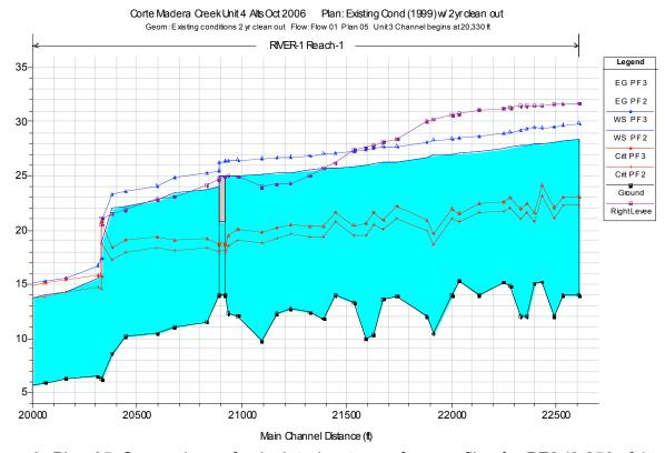
**Figure 1.** Plan 05. Comparison of calculated water surface profiles for PF2 (3,250 cfs) and PF3 (4,100 cfs) in the Unit 4 reach for 1999 existing conditions geometry (g04), including the existing Lagunitas Road Bridge configuration.
